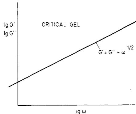
**Figure 2.** Same as in Figure 1, at the critical extent of reaction. The power law extends throughout the entire frequency range.
