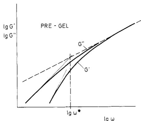
**Figure 1.** Schematic plot of the frequency dependence of the real and imaginary part of the dynamic modulus in the pre-gel state. Above the crossover frequency  $\omega^*$  the typical behavior is a power law (here  $\omega^{1/2}$  for a stoichiometrically well-balanced system, dashed line), while below  $\omega^*$  typical liquid behavior is present.
