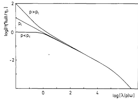
**Figure 6.** Frequency dependence of the dynamic viscosity as given by eq 4.8 for  $p < p_c$  and eq 4.20 for  $p > p_c$  in rescaled units. The ratio  $L/l$  was chosen to be 100; the spectral dimension  $d_s$  is  $4/3$ .
