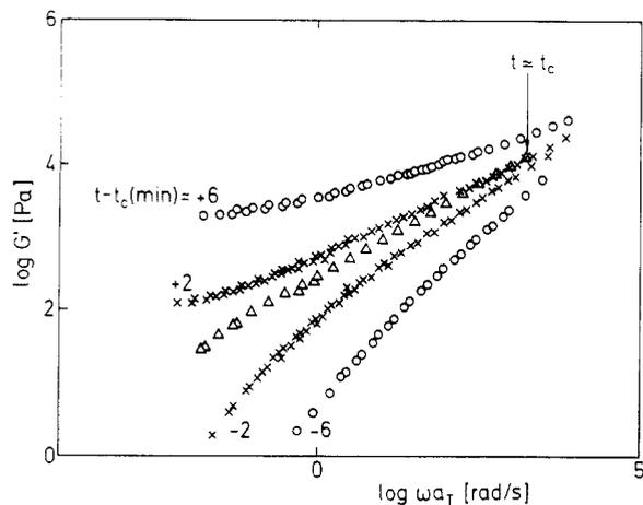
**Figure 4.** Experimental result.<sup>12</sup>  $t$  is the reaction time, before the cross-linking reaction is stopped by poisoning the catalyst.  $t_c$  is the gel time, corresponding to the critical extent of reaction  $p_c$ .
