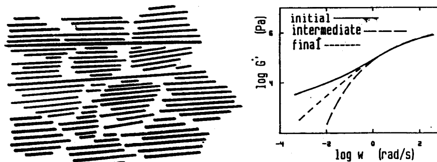
Fig. 14. Healing of grain boundaries during annealing.
