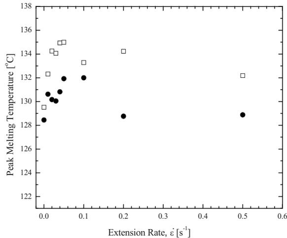
**FIG. 9.** Peak melting temperature as a function of extension rate for isotactic poly-1-butene samples at  $T_c=98^{\circ}C$ . Included are the solutions for DP0401M ( $\square$ ) at a fixed strain of  $\epsilon=5.0$  and PB 0200 ( $\bullet$ ) at a fixed strain of  $\epsilon=4.0$ .
