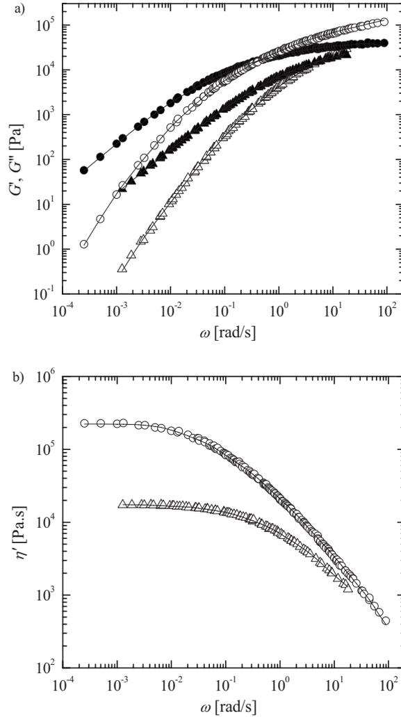
**FIG. 2.** The oscillatory shear master curves of DP0401M ( $\Delta$ ) and PB0200 ( $\circ$ ) for a temperature of  $T_c=98^\circ\text{C}$ . Included in (a) are the solutions of modulus master curves with storage modulus  $G'$  (open symbols) and loss modulus  $G''$  (filled symbols), while (b) includes complex viscosity master curves. Superimposed over both sets of data are solid lines representing the multimode Maxwell fits to each data set.
