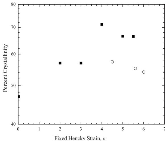
**FIG. 10.** Percent crystallinity as a function of series of strains for isotactic poly-1-butene samples. Included are the solutions for DP0401M at a fixed extension rate of  $\dot{\epsilon}=0.05 \text{ s}^{-1}$  (■) and  $\dot{\epsilon}=0.5 \text{ s}^{-1}$  (○).
