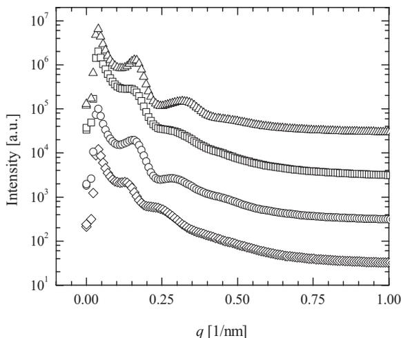
**FIG. 8.** Intensity of the scattering images presented in Fig. 7 as a function of scattering vector,  $q$ , for DP0401M. Included are results for the case of quiescent crystallization ( $\diamond$ ) and crystallization following stretches of extension rates of  $\dot{\epsilon}=0.01 \text{ s}^{-1}$  ( $\circ$ ),  $\dot{\epsilon}=0.05 \text{ s}^{-1}$  ( $\square$ ), and  $\dot{\epsilon}=0.5 \text{ s}^{-1}$  ( $\triangle$ ). All stretches were performed to an accumulated strain of  $\epsilon=5$ .
