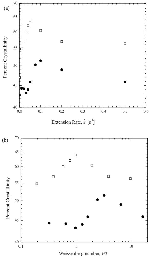
**FIG. 5.** Percent crystallinity as a function of (a) extension rate and (b) Weissenberg number for isotactic poly-1-butene samples at  $T_c=98^\circ\text{C}$ . Included are the solutions for DP0401M ( $\square$ ) at a fixed strain of  $\epsilon=5.0$  and PB 0200 ( $\bullet$ ) at a fixed strain of  $\epsilon=4.0$ .
