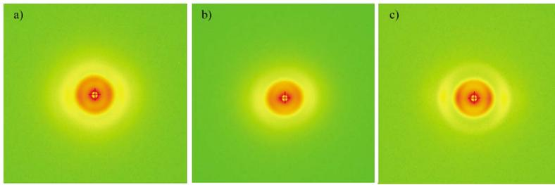
**FIG. 7.** Two dimensional small angle x-ray scattering patterns for DP0401M samples crystallized following stretches of extension rates of (a)  $\dot{\epsilon}=0.01 \text{ s}^{-1}$ , (b)  $\dot{\epsilon}=0.05 \text{ s}^{-1}$ , and (c)  $\dot{\epsilon}=0.5 \text{ s}^{-1}$ . All stretches were performed to an accumulated strain of  $\epsilon=5$ . The stretch direction is aligned horizontally to the scattering patterns.
