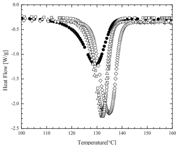
**FIG. 4.** A pictorial representation of DSC fits with heat flow as a function of temperature. Included are the solutions of PB 401M samples with extension rates  $\dot{\epsilon}=0.01 \text{ s}^{-1}$  ( $\square$ ),  $0.04 \text{ s}^{-1}$  ( $\diamond$ ),  $0.5 \text{ s}^{-1}$  ( $\triangle$ ) all at a fixed strain of  $\epsilon=5$ , and an unstretched sample ( $\bullet$ ).
