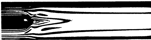
Fig. 7. Birefringence pattern for LDPE at 160°C with an average outlet velocity of 0.8 mm/s.
