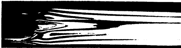
Fig. 9. Birefringence pattern for LDPE at 160°C with an average outlet velocity of 1.6 mm/s.
